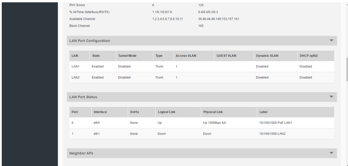
FIGURE 142 Viewing an AP's Ethernet port configuration
