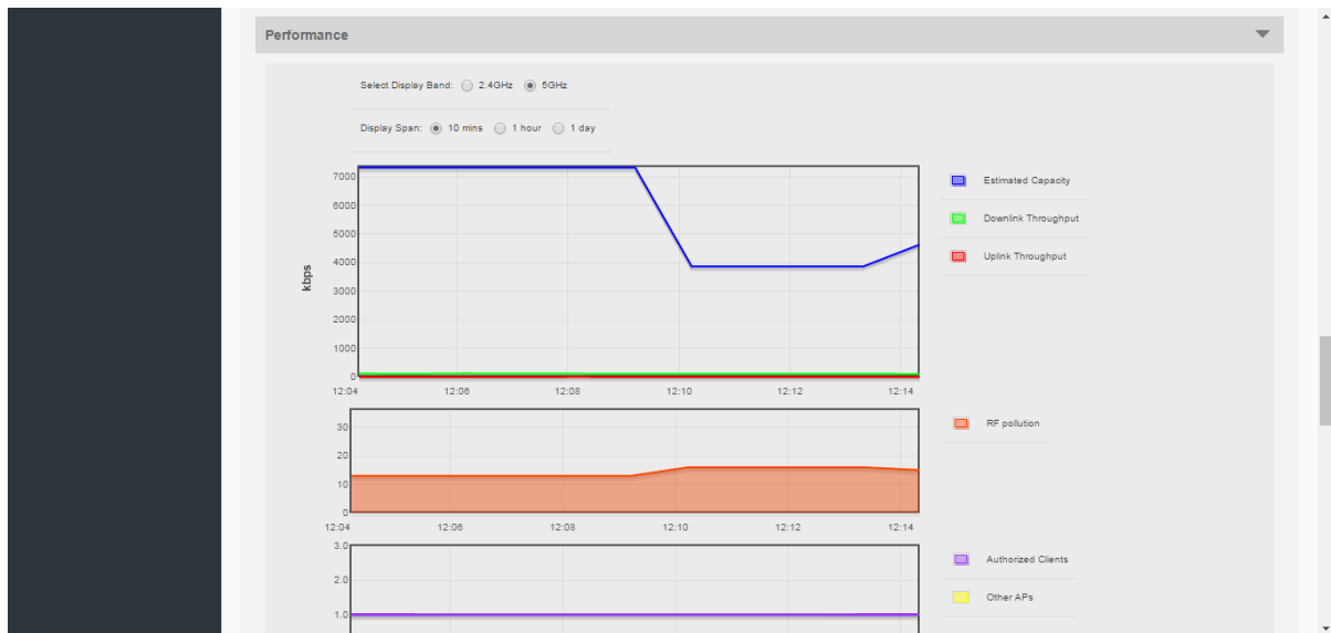
FIGURE 203 Monitoring an AP's performance
